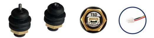
Housing body: Friction lock PCB header: JST: BMO4B-GHS-TBT(LF)(SN)(N) Mating wire harness: 10" 28AWG PTFE to five position connector housing: JST GHR-04V-S
