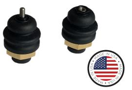
The TSD Series is a micro, multi-axis Hall effect joystick purposely designed for uncrewed systems and robotics applications. Available with choice of M3 male or M2 or M3 female threading, the TSD Series allows users to easily adapt their own handle. The TSD Series is rated for over 2.5M actuations and features IP67 above panel sealing as standard.
